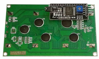
It is LCD with 20-Character 4-Line, blue BACKLIGHT and white font (STN NEGATIVE BLUE). The display is I2C Interface that saves amount of I/O of CPU when connecting with LCD. It provides example program for using with Board Arduino; for example, connecting to I2C Boards from ETT directly like ET-ESP8266-RS485, ET-MEGA32U4-RS485 and etc.
